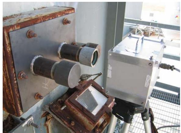
**b) Collimator and Scanner Enclosure**
