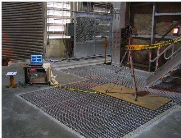
Fig. 2. Detector mounted on a tripod at right, receiving signals from a laser beam passing out of the regenerator section of a float glass furnace. The LTS-100 processing unit can be seen on the left.
